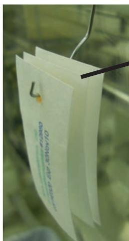
Plastic spacers have been placed on the wire hanger between each BI to ensure proper vapor flow around each BI unit.
