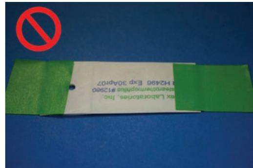
Figure 3. Examples of IMPROPER BI configurations when using adhesive tape
