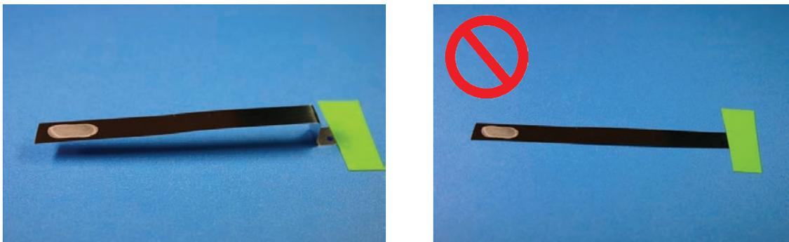
**Figure 5. Examples of proper (left photograph) and improper (right photograph) BI configurations**
