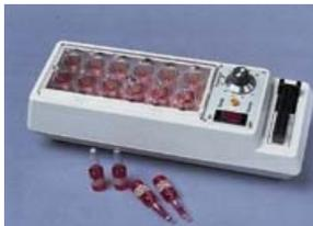
A small table top incubator can be purchased that will hold up to 12 ampoules at one time. The incubator is preset for temperature and the ampoules are easily visible to monitor for color change. After 48 hours of incubation, if no color changes occur, the ampoules can be removed and disposed of.
