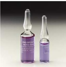
There is an easier method, there are sealed glass ampoule type BIs designed specifically for such cycles where liquids are going to be present. These glass ampoules contain the same spores that would be used on a spore strip and they also contain the growth media that would be in the tube that a spore strip is transferred to. Therefore the need to aseptically transfer to growth media is eliminated. One simply inserts the ampoule into the bag being sterilized and upon
