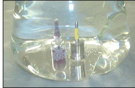
Figure 3: BI Ampoule and Logger in a flask
